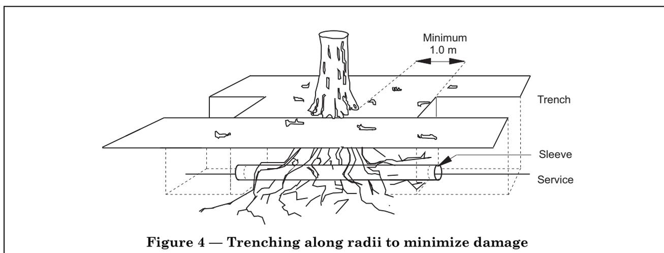
**Figure 4 — Trenching along radii to minimize damage**
