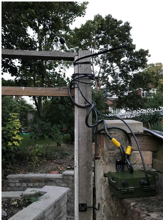
Figure 3.1 Static detector installed on fence line between gardens
