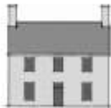
i) Relationships of window to wall - correct The diagram shows a ratio of approximately 15%
